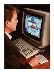
offers software drivers for two kinds of speed control — relative and absolute. Relative mode features automatic acceleration already familiar to mouse users. Move your finger slowly for pixel-by-pixel control or move it quickly to accelerate across the screen. Better still, absolute mode is even quicker — the tablet's 1,000 by 1,000
